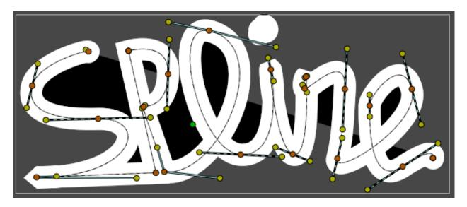
Fig. 1: A spline of "Spline". Can see orange vertex and yellow tangent *Handle*
